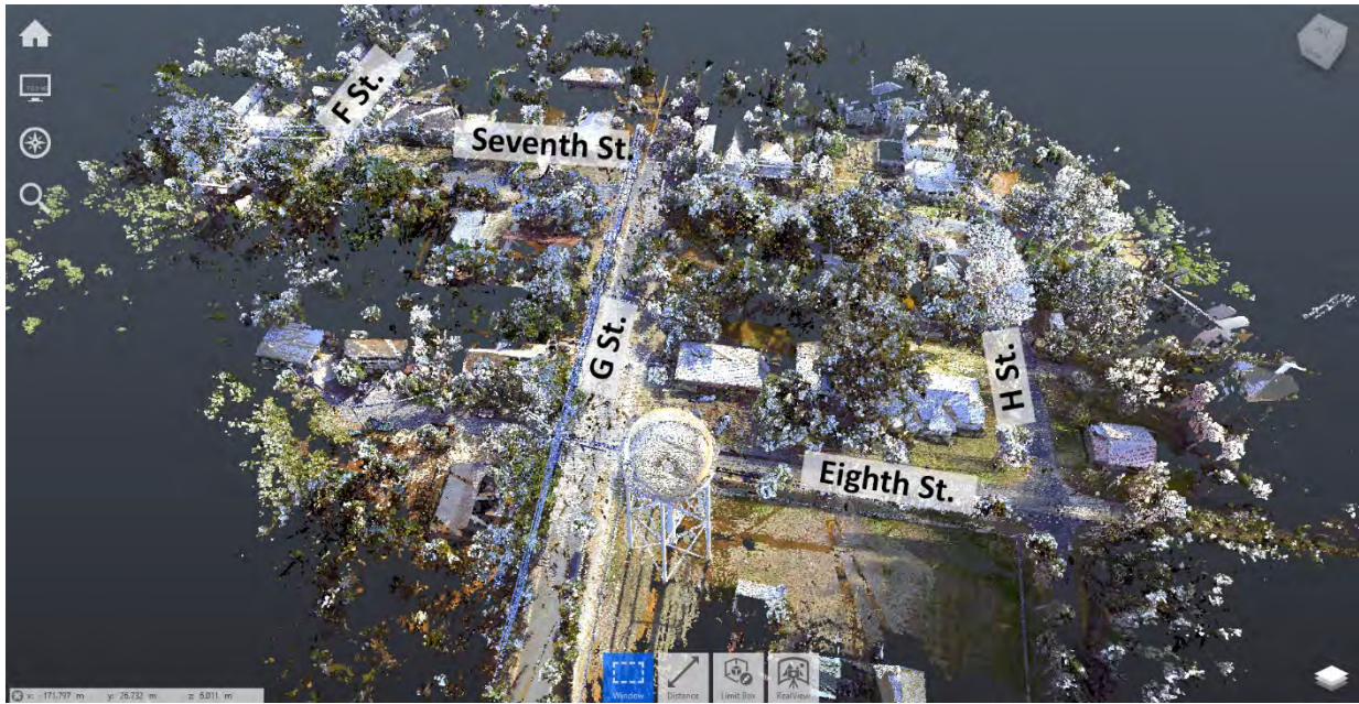
Figure 4. Laser scan point cloud aerial view, looking southwest.
